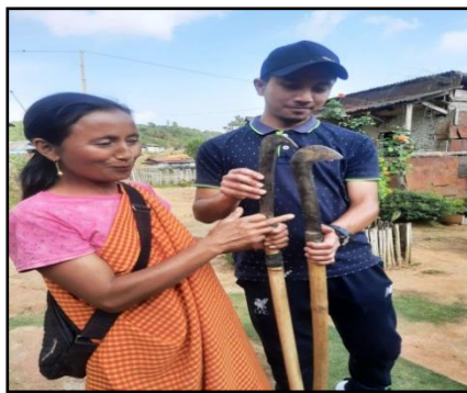
Fig. Dao with long handles (the lighter one for cutting grass and the heavy one for cutting fire woods).
